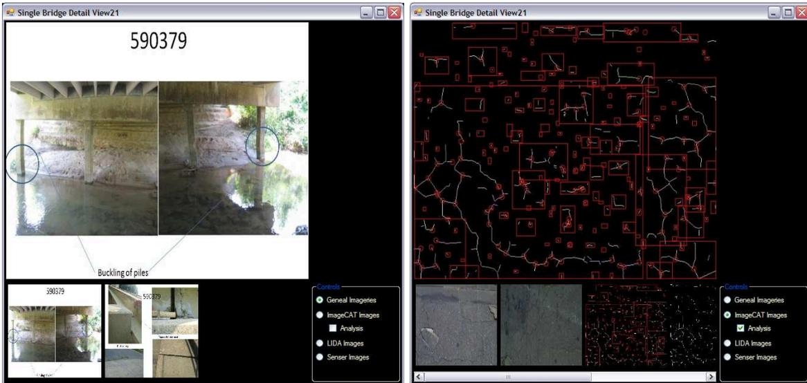
Figure 5. Left: (A)The Details collected from field inspection. We could easily see the supporting structure for this bridge is severely bent. Right: (B) The Analysis Results from ImageCAT Inc.?
