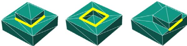
**Figure 8:** Three edge types highlighted in yellow. Left – concave. Middle – convex. Right – planar.
