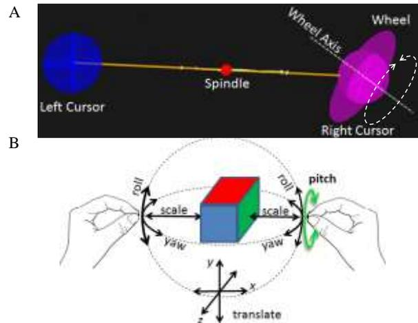
**Figure 3: Spindle+ Wheel condition. (A) Spindle+Wheel’s visual feedback. (B) Bimanual DOF’s of Mapes and Moshell “5DOF+Scale” technique [9] versus “Spindle+Wheel” [4] which adds pitch (green).**
