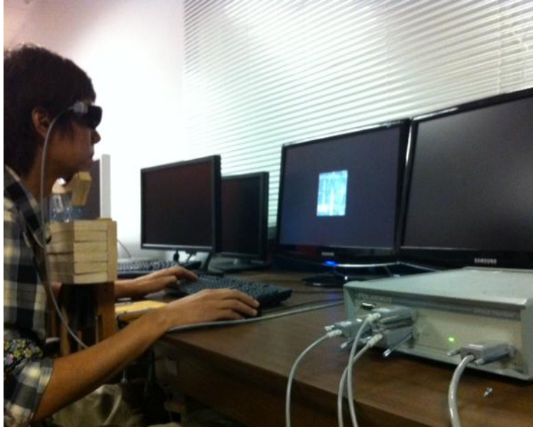
Figure 2: Environment system: This picture shows our environment system. A 3D display with Nvidia 3D vision shutter glasses, Polhemus tracker and a chin-rest.
