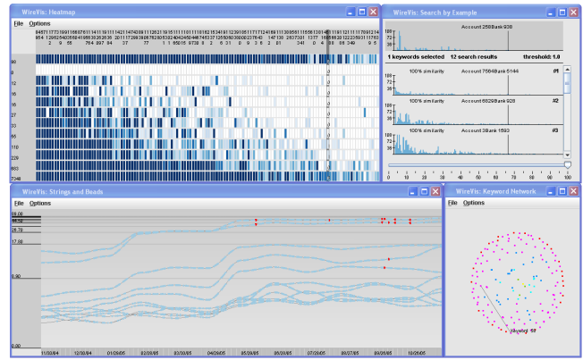
Figure 1: Overview of WireVis. It consists of four views including a heatmap view (top left), a time-series view (bottom left), a search by example view (top right), and a keyword relation view (bottom right).
