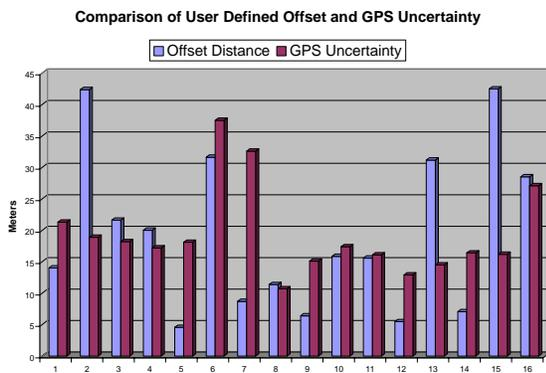
Figure 11 – Distance between the offset and GPS position is typically more than 10 meters
