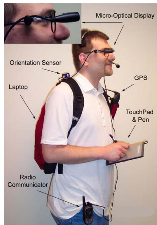
Figure 1 - User with GPS Tracker, Orientation Sensor, Radio, Eye Display, and Touchpad
